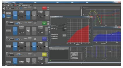
In addition, the easy-to-use hd LevelZ PC Remote Software provides even more detailed information on individual requirements and an unlimited number of user presets and configurations.
