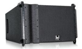
hd LSA12 LineSourceArray Module The hd LSA12 is an efficient LineArray element of the latest generation, equipped with a specially designed high performance 12" neodymium low frequency chassis. The high frequency unit is equipped with two 1.4" neodymium compression drivers with special polymer diaphragm coupled to dedicated line source wave formers to generate a cylindrical wave front.
